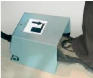
Sheet clamps are operated by a foot switch, which can be located freely.
