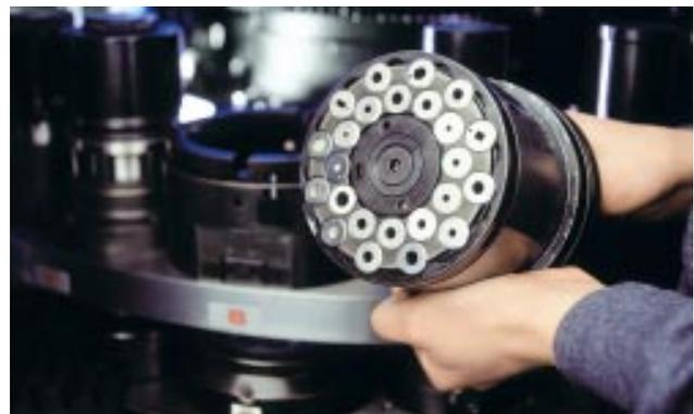
The turret can be equipped with **MultiTool® stations** to increase the number of tools. The MultiTool® station is mounted on the turret like a normal tool station and the tools are mounted in rapidly changeable punch and die cassettes, which are available also as additional equipment.
