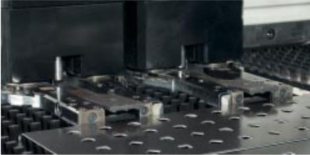
The clamps are equipped with sheet detecting sensors, which continuously monitor sheet security in the clamp, ensuring accuracy and reliable machine operation.
